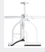
Non-rising handwheel with indicator DN200 - DN350 8" - 14"
